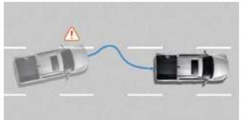
Lane Departure Warning (LDW) Warns the driver whenever the vehicle begins to move out of its lane unless the directional indicators are on in that direction.
