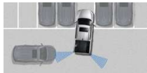
Rear Cross-Traffic Alert (RCTA) Assists the driver when backing up by detecting the presence of vehicles approaching on either side in the rear.
