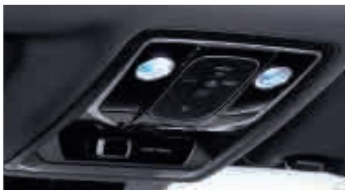
Overhead console, Touch switch room lamp, Seatbelt Reminder
