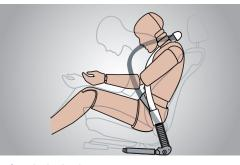
**Safety belt dual pretensioner** Pre-tensioning mechanism greatly reduces the risk of serious injury.
