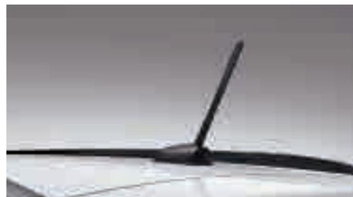
Roof-mounted pole antenna
