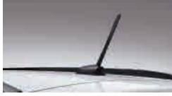
Roof-mounted pole antenna
