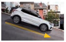
**Hill Descent Control (HDC)** Activating HDC on extremely steep hills automatically shifts the vehicle into low gear and begins brake pumping action for a safe descent.
