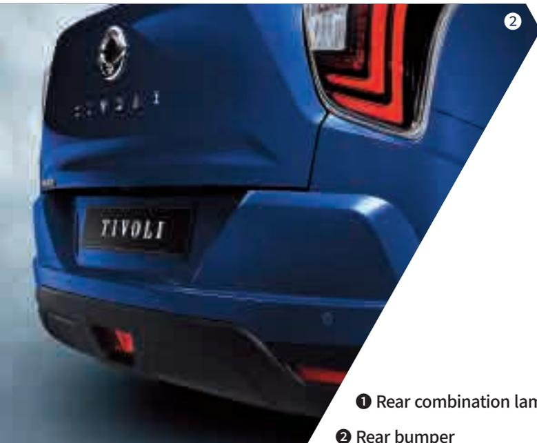
❶ Rear combination lamp with LEDs
